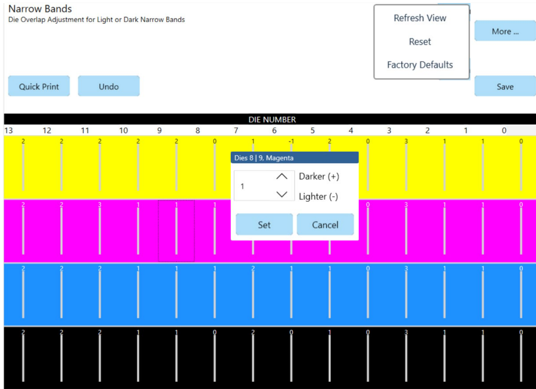
Figure 8-27. Die Alignment for Narrow Bands
