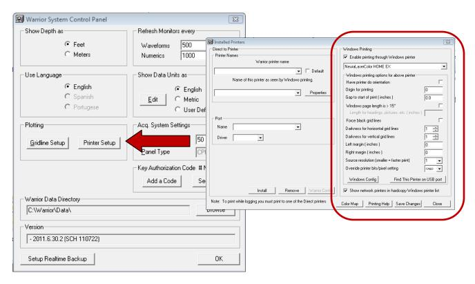
Neuralog printers use the **Windows Printing** side of the Installed Printers Dialog. Neuralog printers do not use any parameters on the **Direct to Printer** side of the Dialog.
