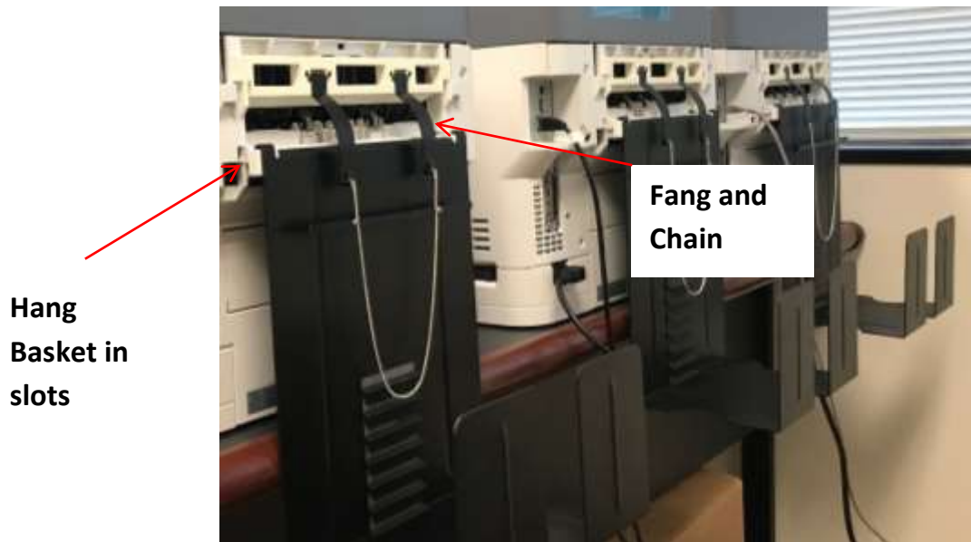
Figure 2-8. Installing the Paper Stacker
